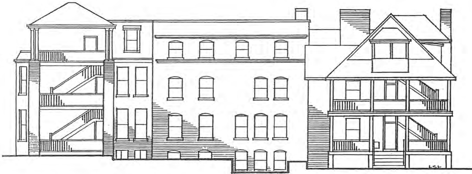
1992 south elevation of No. 87 as seen from Oxford St. At right, Fuller's roughcast home of the 1860s with an 1890 front and entirely brick-veneered. For subsequent additions see p. 19. (Stephen Langmead, architect)
